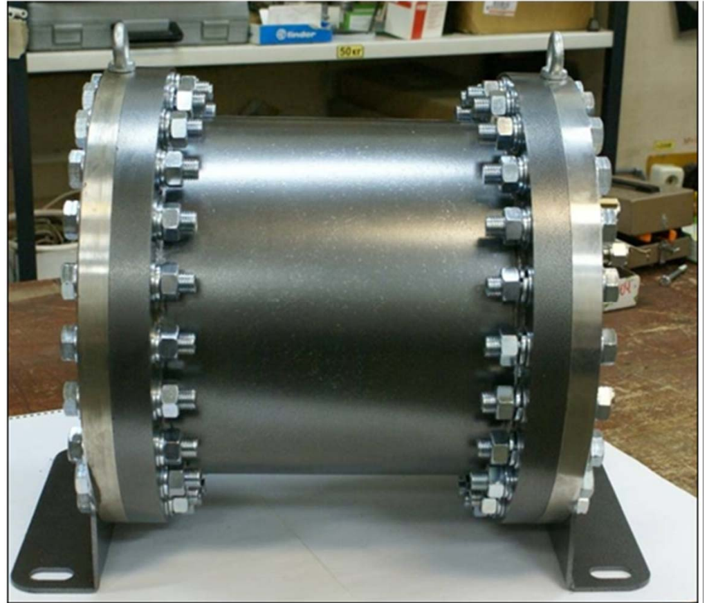
Bipolar modulus for electrolysis at 130 bars
