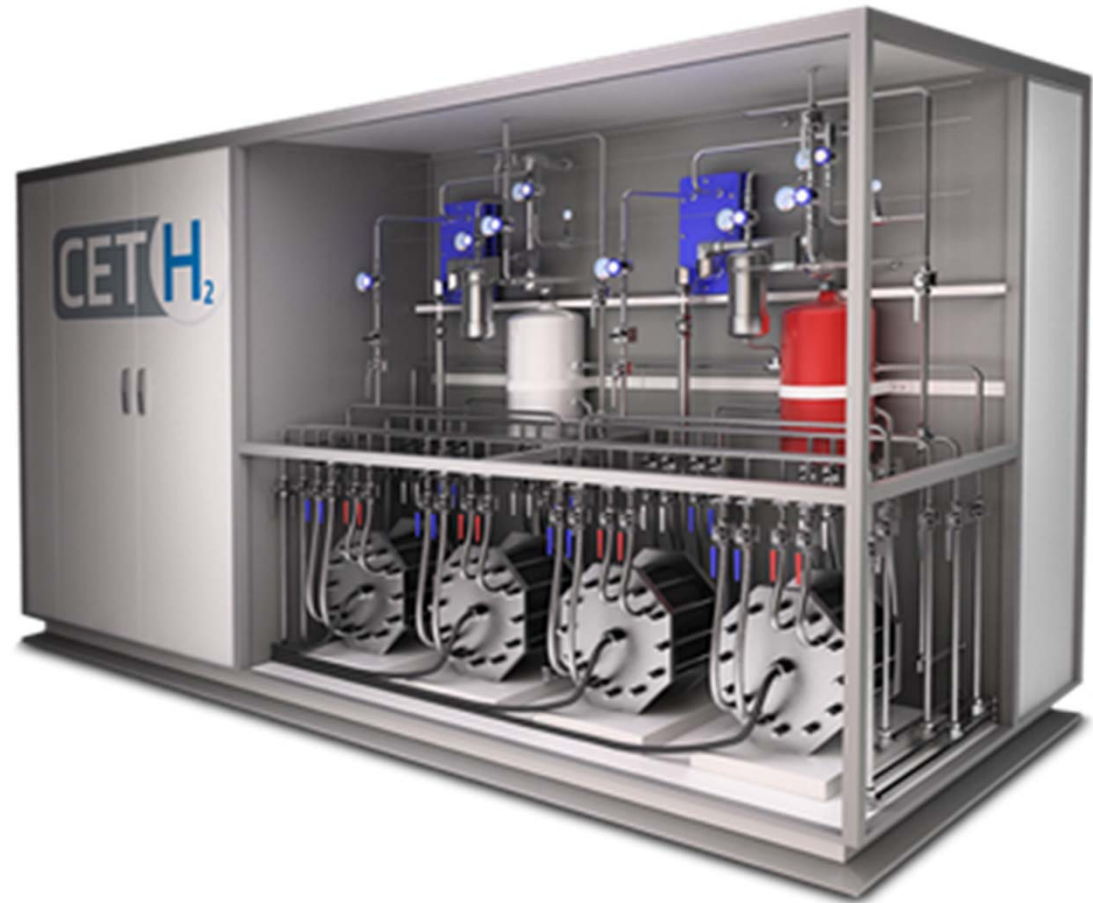
4-modules for water electrolysis (60 Nm 3 /h H 2 each) : 1.2 MW 14 bars, feeding with tap water at 35°C, 3-5 bars
